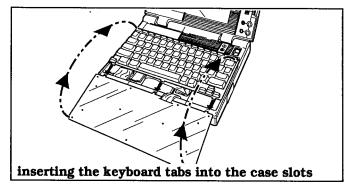
**2.** Hold the front of the keyboard in place while you lower the rear of the keyboard onto the computer case.
